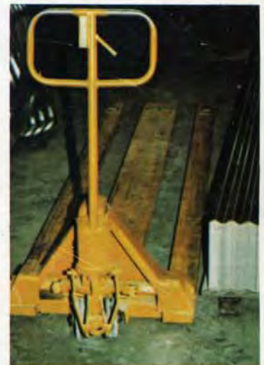
10,000 lb. capacity trucks designed for U.S. Aluminum & Steel Highway Products Co., one of which is a three fork truck.
